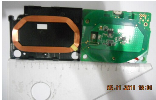
Fig. 9. Practical reader with a transmitting coil.
